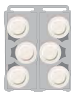
6 columns - plates of \varnothing 118 -230 mm
