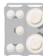
5 columns - plates of \varnothing 102 mm 2 columns - plates of \varnothing 334 mm
